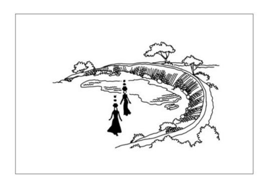
Johad is the name given to small earthen check dams. Due to the extreme heat and desert conditions in Rajasthan, rainwater is harvested in these tanks. Johads are formed when semi-circular mud barriers are built across slopes to catch the monsoon run-off. The rainwater is harvested in these tanks and held for agriculture.
